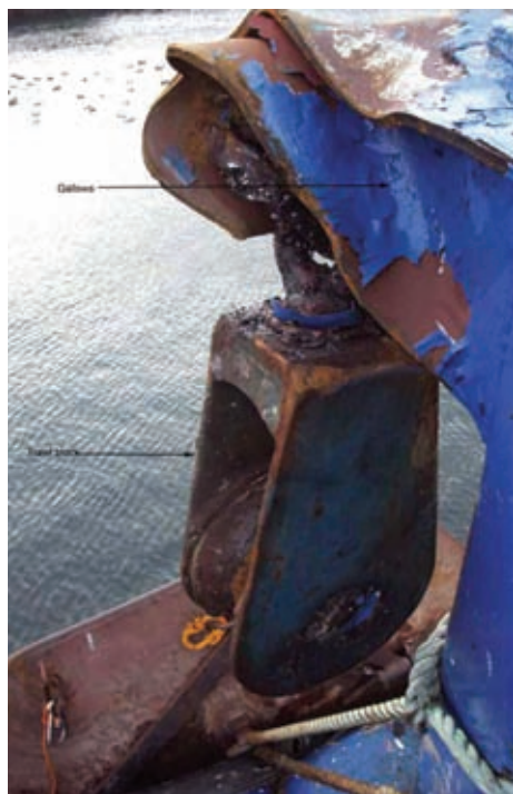
Damage sustained to gallows and trawl block of fishing vessel. Photo: MAIB
